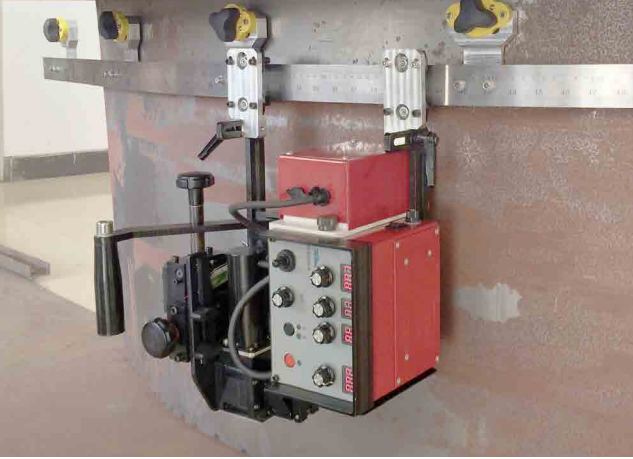
Tractor drive on Flexible steel-rail
