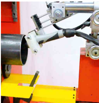
Also for internal welding
