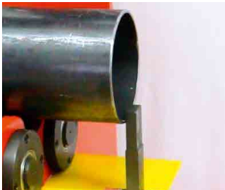
Pneumatic limit stop
