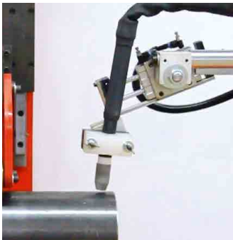
pneumatic torch holder and stand
