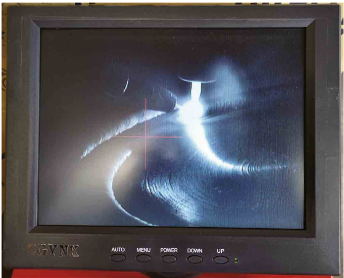
Pulse TIG with filling
