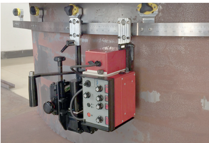
Tractor drive on Flexible steel-rail
