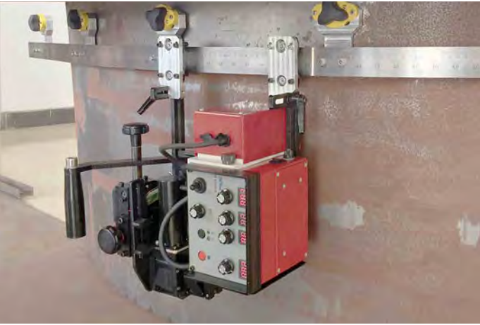
Tractor drive on Flexible steel-rail
