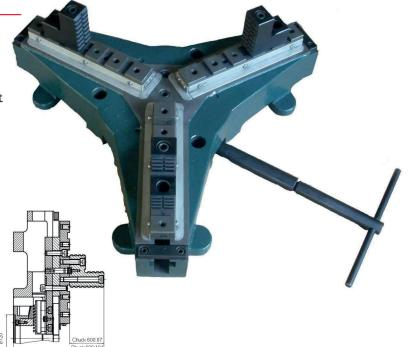
The jaw chuck of this series fit without modifications to the JAVAC rotary tables with three and six grooves.
