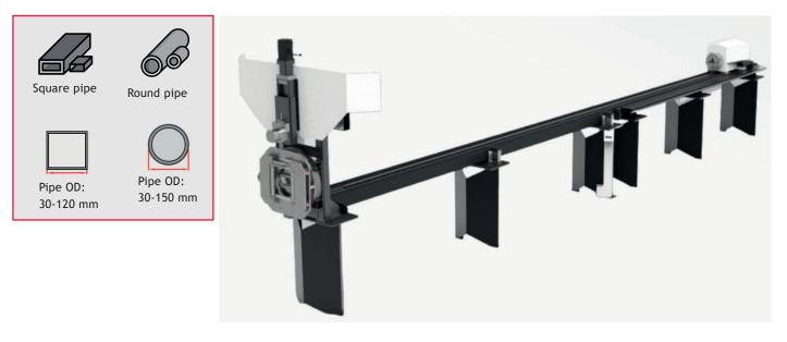
Fully machined rail and rack positioning, Machine mechanism precision smaller than 0.02mm to promise cutting precision.
